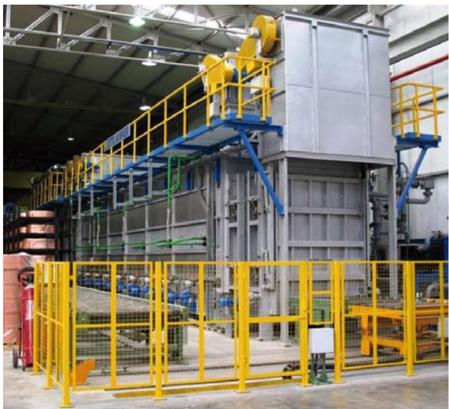
Exit end of a roller hearth furnace
