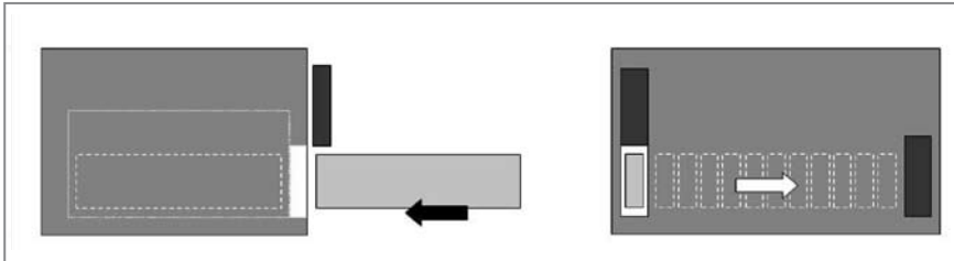
SLE Pusher Furnace®: Left: front view with side door. Right: side view with open entry door and closed exit door.
