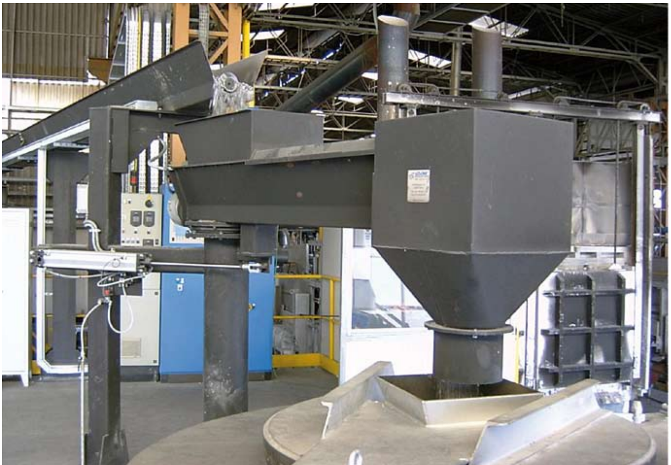
Example of a coreless induction furnace plant for the melting of fine-grained material
