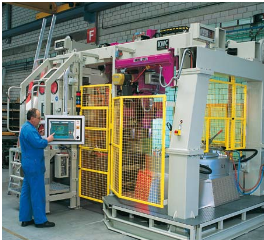
INDUGA-KWC-Low-pressure die casting line
