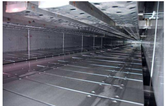
Interior view of the furnace with jet heating nozzle beams, dual-track conveyor, independent track control
