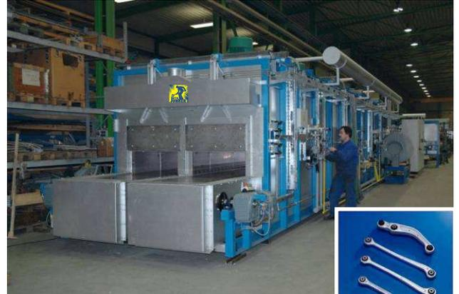
Heating of cast automotive suspension parts for a downstream forging operation (COBAPRESS® process), loading side
