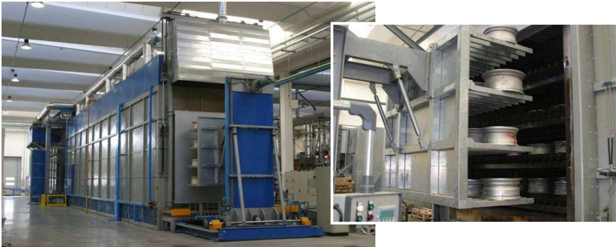
Heat-treatment system for solution annealing and artificial ageing of cast aluminium alloy wheels
