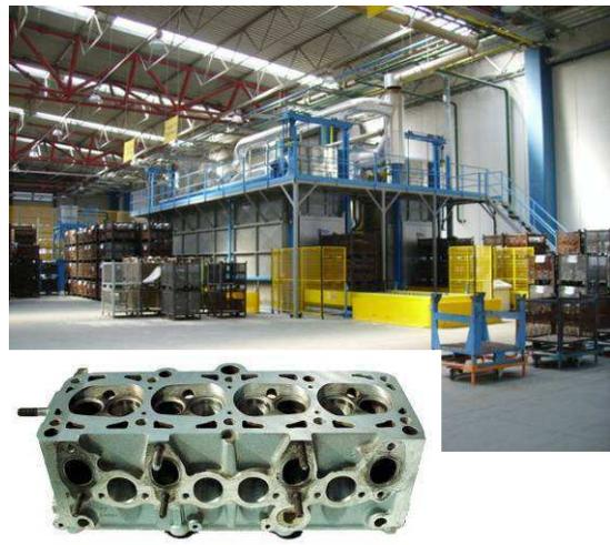
Each furnace has its own conveyor system. The two doors can be opened independently of each other to prevent excessive cooling of the furnace during loading and unloading operations (chimney effect).
