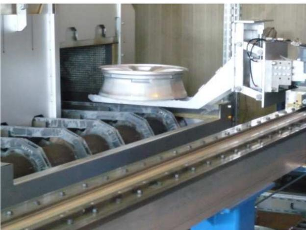
Loading operation by means of a manipulator
