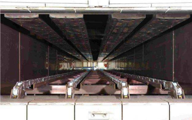
Interior view of the solution annealing furnace; two tracks; all-internal chain conveyor
