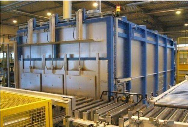
Wheel heating furnace before flow forging
