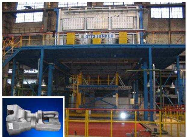
Examples: Drop-bottom furnace systems for solution annealing large forgings for the aircraft industry. Direct electric heating, stationary water quench in a pit, charging car serving as load and unload station and for charging the furnace.
